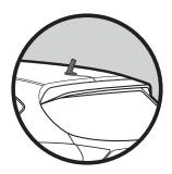
**SUV/Van/Hatchback:** Cable routed into top of hatchback door.
