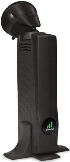
Mount booster in the center of your inside back window using one of the two options below. We suggest using the adjustable window mount option for vertical or near-vertical windows and the adhesive base mount for windows that are more angled, like sedans. For both installations you need to place the booster as close to the rear window as possible. For best performance, be sure the booster is mounted vertically with the SureCall logo facing the front of the vehicle.
