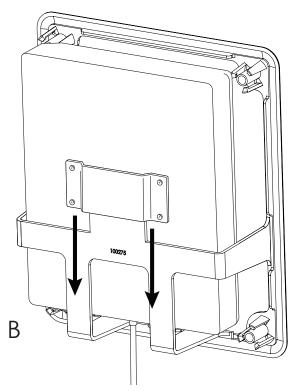
1. Locate an area on the wall where the In-Wall Antenna Bracket will be installed. The size of the hole to be cut into the wall should be 8-1/8" horizontal by 9-1/2" vertical. (See template on back)
