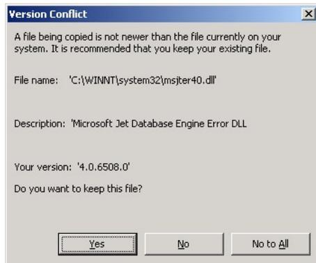
The displayed message prompts you to select whether to save the newer version, or replace it with the installed component. Press **Yes** to keep the newer version' or **No** to replace it. You can also select **No to All**, in order to define that each time the installer encounters a newer file it will be replaced.
